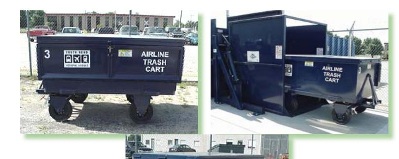
The Towable Steel Waste Carts have a low loading height, due to fold-down side gate. With special 16" diameter extra heavy duty solid pneumatic rubber wheels, tapered bearings and a hinged lid that opens when the cart is in the dump position, you have a 5th wheel steel trailer of a very practical and rugged design.
