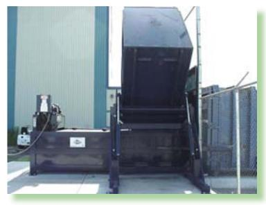
The above photo features a Model 8260-S-2-6 Compactor with right hand side load hopper, and Model HP-3000 hydraulic Cart Dumper
