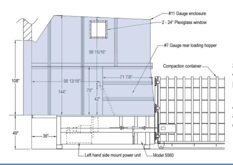
Side view showing a 144" high x 96" wide total enclosure with built-in hopper.
